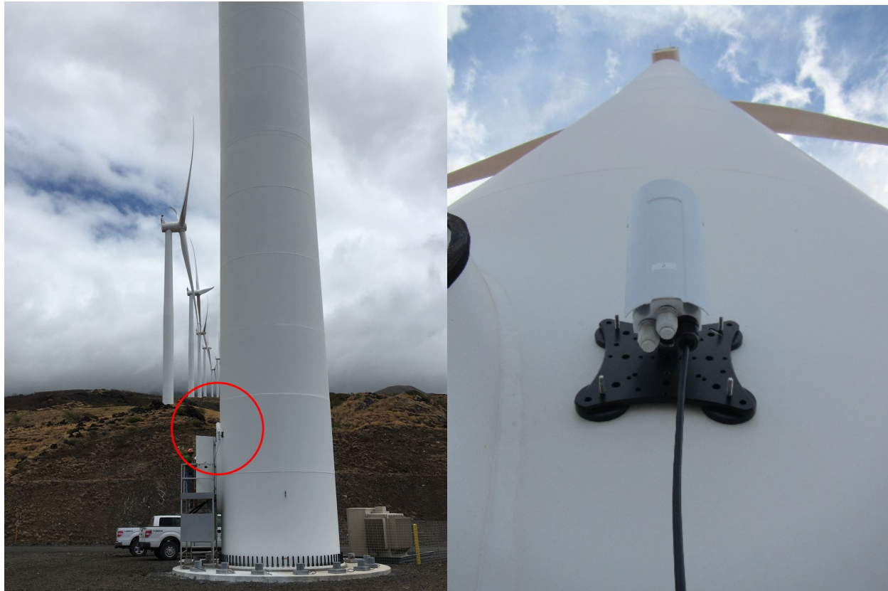
Figure 1. Placement of camera on turbine monopole (circled, left panel) and camera orientation (right panel).
