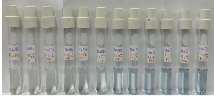
Figure 3: Heteropoly blue color complex formation across phosphate concentrations ranging from 1 \times 10^{-7} \text{M} to 1 \times 10^{-5} \text{M} \text{NaH}_2\text{PO}_4 solutions containing \text{NaOH} ( 1 \times 10^{-3} \text{M} ).
