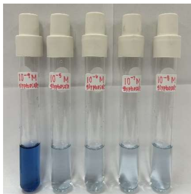
Figure 5: Heteropoly blue color complex formation across glyphosate ( 1 \times 10^{-8} to 1 \times 10^{-4} \text{M} ) samples that were subjected to 15min of ozone gas. Samples also contained 1 \times 10^{-3} \text{M} \text{NaOH} .
