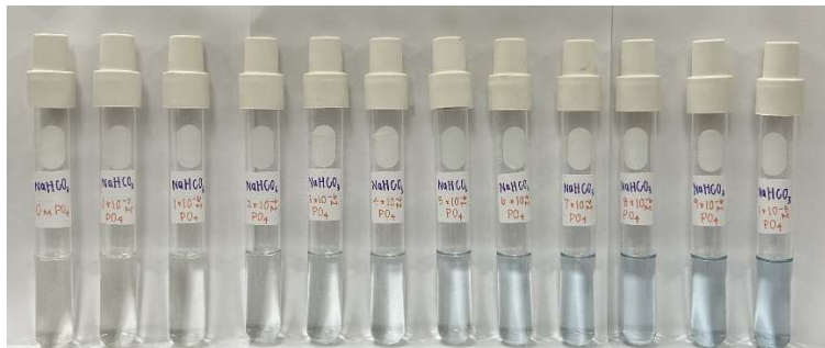
Figure 4: Heteropoly blue color complex formation across phosphate concentrations ranging from 1 \times 10^{-7} \text{M} to 1 \times 10^{-5} \text{M} \text{NaH}_2\text{PO}_4 solutions containing \text{NaHCO}_3 ( 1 \times 10^{-1} \text{M} ).
