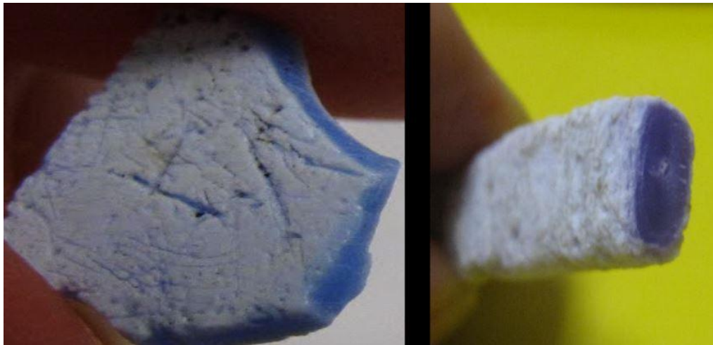
Figure 4. Outside weathering was marked as present or absent for all polyethylene (PE) and polystyrene (PS) beach samples. The images above are examples of samples that were marked present for outside weathering. A sample was marked present for outside weathering if the surface of the plastic sample had visible yellow or white discoloration.
