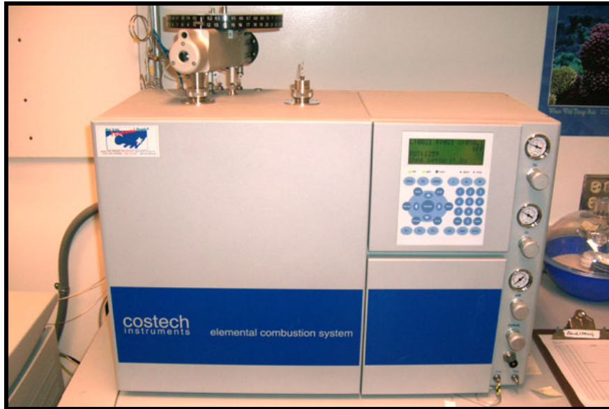
Figure 5. The University of Hawai'i at Hilo Elemental analyzer used to volatilize fish muscle tissue samples for isotope analysis.
