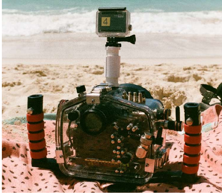
Figure 2. Dual camera rig for simultaneous capture of action camera (GoPro Hero4) video and DSLR (Canon EOS 60D) photo capture. The homemade PVC riser mount for the action camera on the top of the housing prevents the dome of the housing to be included in the wide frame of the GoPro Hero4 while allowing simultaneous image collection of the same area.
